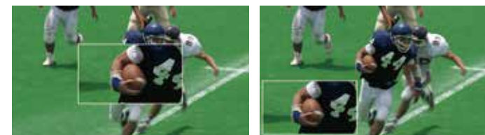
Pixel-to-Pixel display on the VF screen. The display position is selected from the center area and four quadrant area.
