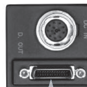
Small SDR (Mini-CameraLink) Connector [24.4 x 9.0 mm]
