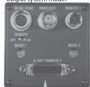
Conventional MDR-26 CameraLink Connector [39.7 x 12.9 mm]
